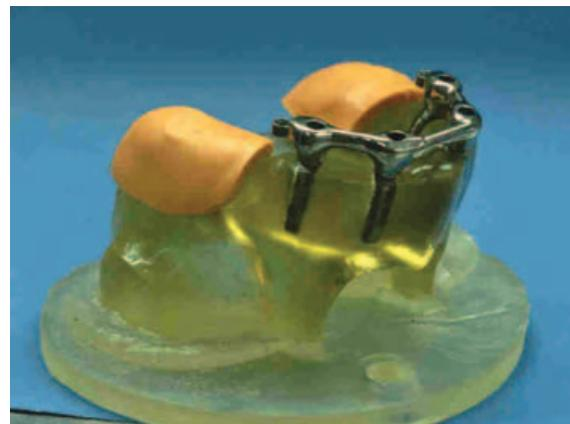
**Figure 1.** Photoelastic model with splinted bar-ERA attachment system.
