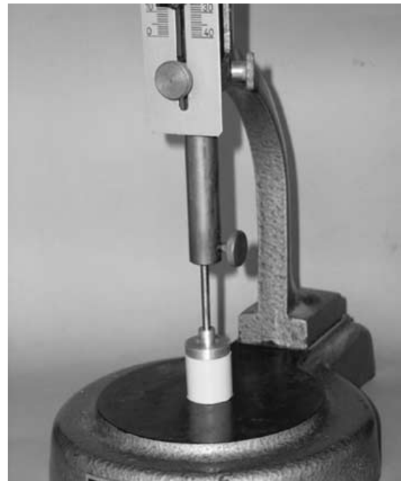
Figure 2. The testing instrument used to exert pressure on the specimens of the interocclusal registration materials.
