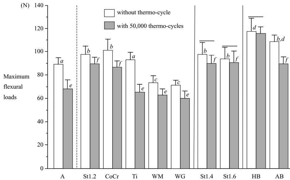
**Figure 2.** Loads required to cause fracture of each flexural specimen. The same letters on columns of the same thermo-cycle number indicate no significant difference ( $p > 0.05$ ). Columns connected with horizontal bars are not significantly different ( $p > 0.05$ ).
