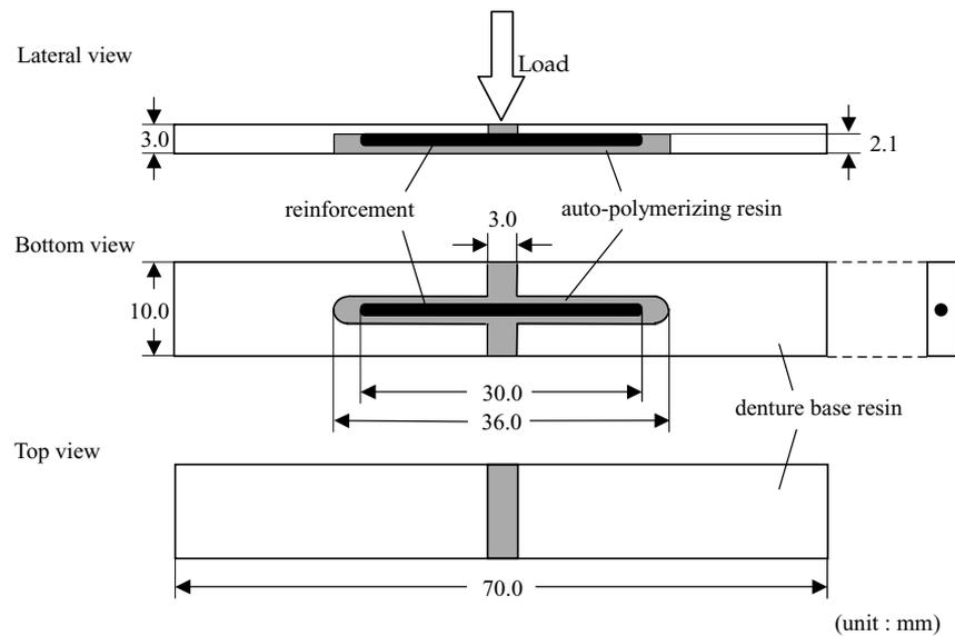
**Figure 1.** Schematic drawing of bending specimen.
