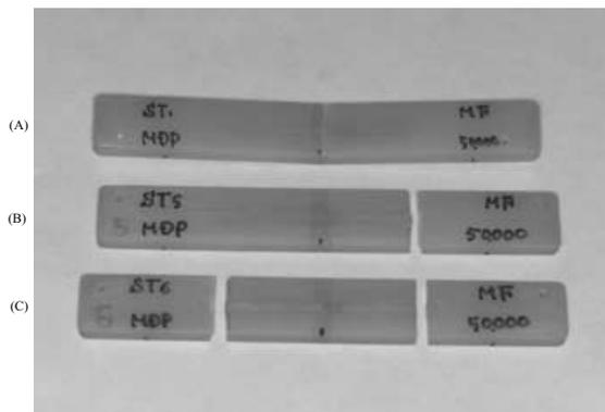
**Figure 3.** Fracture mode after flexural test. Note that fracture occurred at the center on (A) but at the ends of the wire on (B) and (C).
