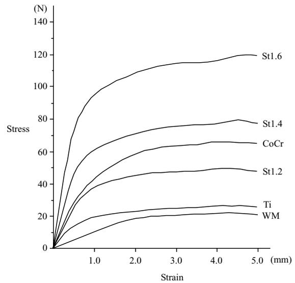
**Figure 4.** Typical stress-strain curve for each metal reinforcement.
