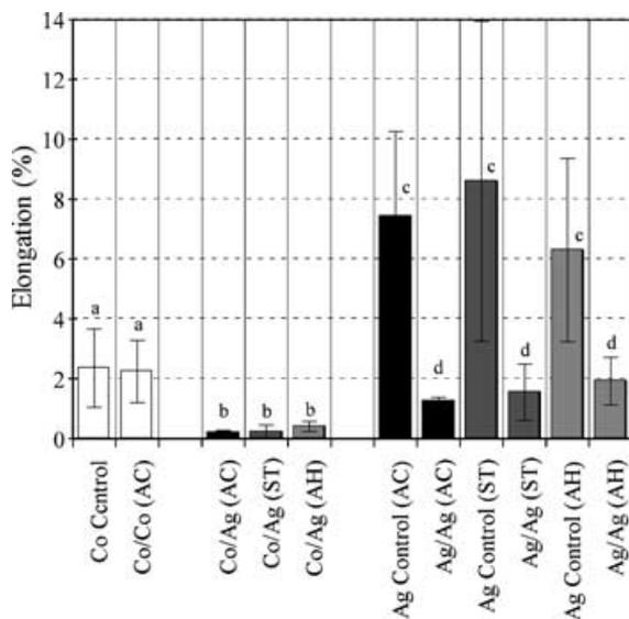
**Figure 3.** Elongation (%) of the specimens. Identical letters indicate no significant differences ( $p > 0.05$ ) in each pairing or among heat treatments.
