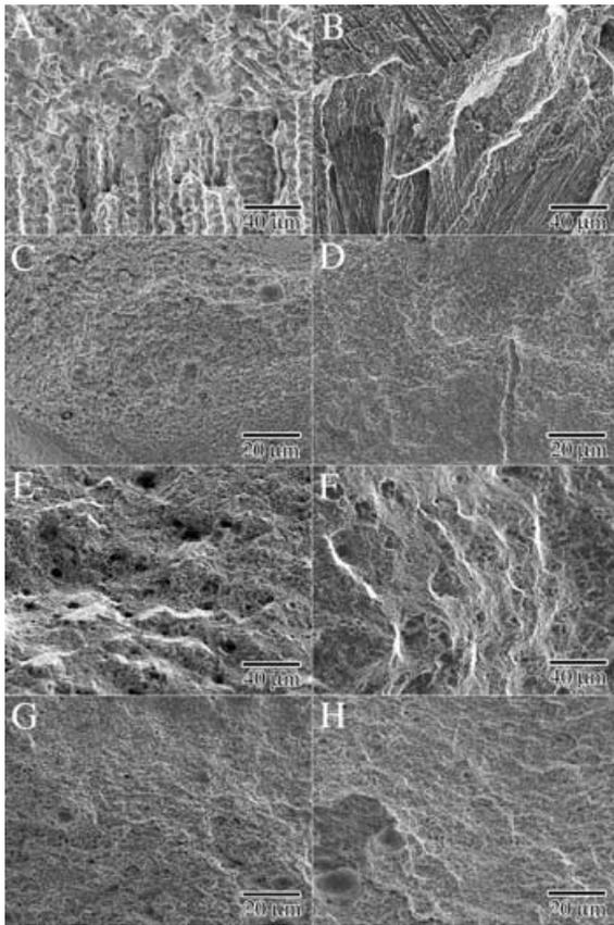
**Figure 5.** SEM micrographs of fracture surfaces of the specimens. (A) Co (Control). (B) Co/Co (Laser). (C) Co/Ag (Laser; AC). (D) Co/Ag (Laser; AH). (E) Ag (Control; ST). (F) Ag (Control; AH). (G) Ag/Ag (Laser; ST). (H) Ag/Ag (Laser; AH).
