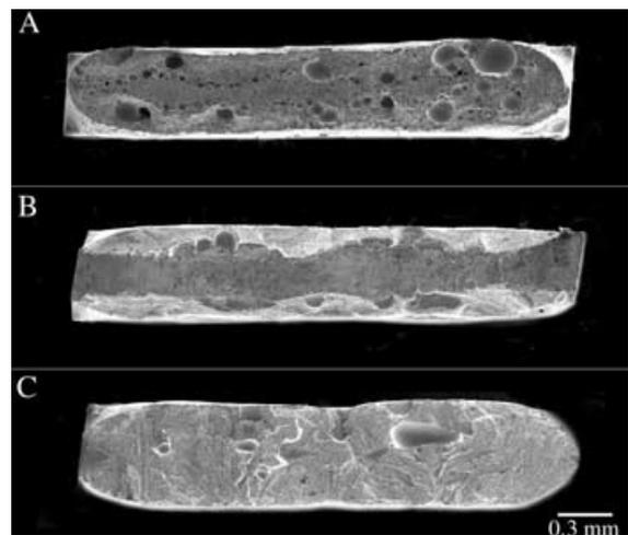
**Figure 4.** SEM photographs of entire fracture surfaces of the specimens. (A) Ag/Ag (Laser). (B) Co/Ag (Laser). (C) Co/Co (Laser).
