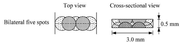
**Figure 1.** Laser-welding configurations used.
