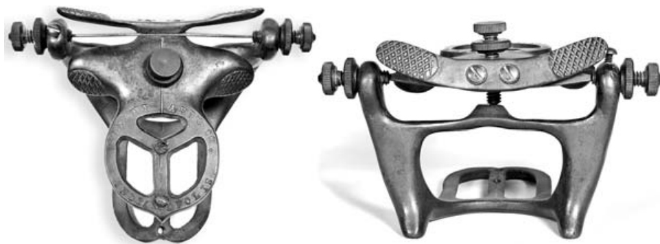
Figure 2. The Stanley "Anatomical Articulator and Grinder," 1924 (Top and back views). The Stanley had both thumb plates and opposing plates for the forefingers, which likely provided better control. A heavy band spring condylar axle was the resistance.
