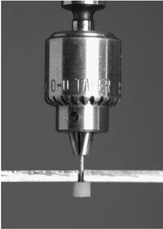
**Figure 2.** The specimen is placed in a fixture on the Universal testing machine with the dowel head grasped with a Jacob's chuck.
