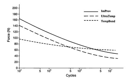
**Figure 1.** Extrapolation of pre-fatigue effects on remaining retention forces for three cements.
