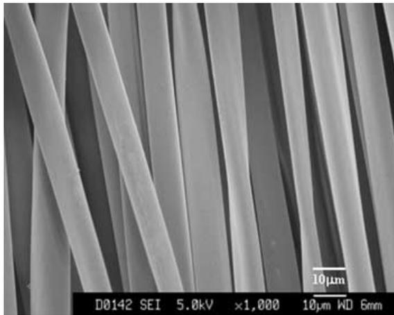
**Figure 2.** FE-SEM image of alumina fiber used as a reinforcement for the alumina-fiber/alumina composite.
