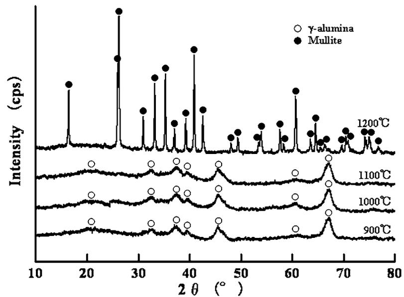
**Figure 7.** XRD patterns of alumina-fiber after sintering.
