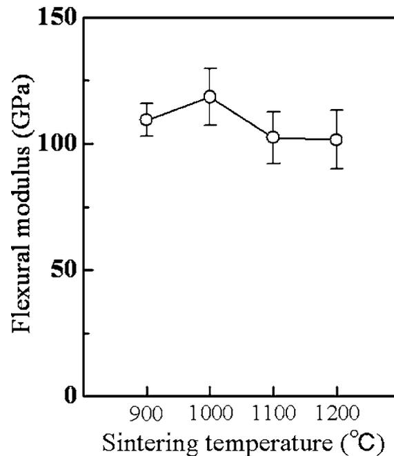
**Figure 6.** Relationship between flexural modulus and sintering temperature.
