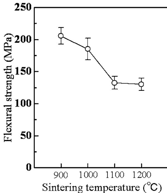
**Figure 5.** Relationship between flexural strength and sintering temperature.
