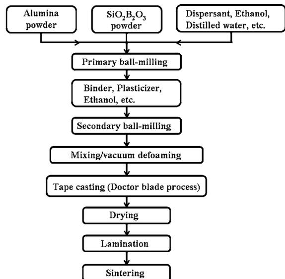
**Figure 1.** Fabrication process of alumina-fiber/alumina composite.
