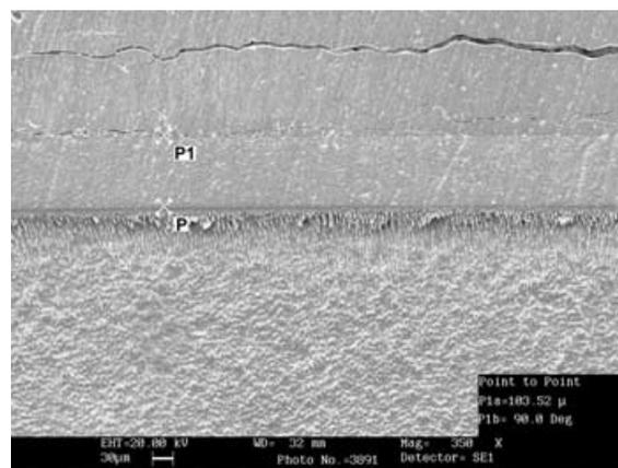
**Figure 1.** Representative sample fabricated with 100- $\mu\text{m}$  spacer (obtained cement thickness P-P1 = 103.52  $\mu\text{m}$ ) (350 $\times$ ).
