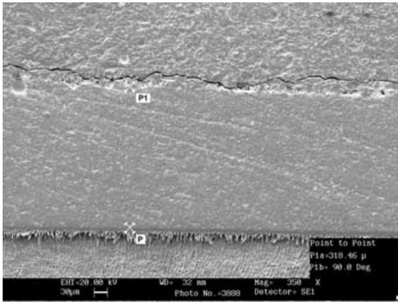
**Figure 3.** Representative sample fabricated with 300- $\mu\text{m}$  spacer (obtained cement thickness P-P1 = 318.46  $\mu\text{m}$ ) (350 $\times$ ).
