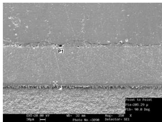
**Figure 2.** Representative sample fabricated with 200- $\mu\text{m}$  spacer (obtained cement thickness P-P1 = 205.29  $\mu\text{m}$ ) (350 $\times$ ).
