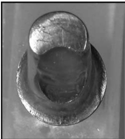
Figure 3. Abutment fully filled with Memosil.
