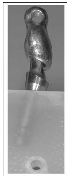
Figure 1. Mounting of implant replica and abutment in acrylic resin with casting constructed on top.
