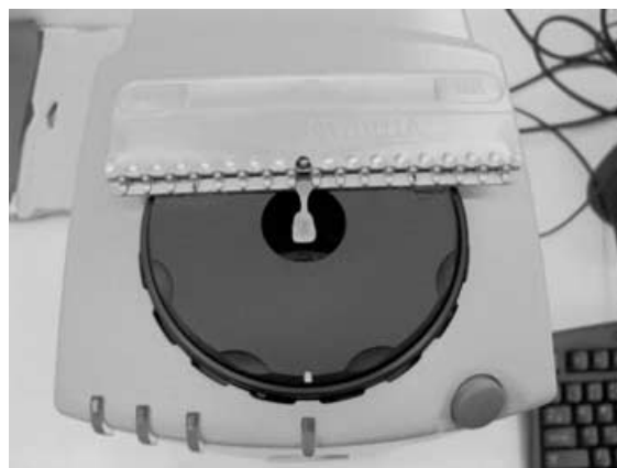
Figure 1. LabScan XE port plate modified by attaching Vitapan Classical Shade tab holder.
