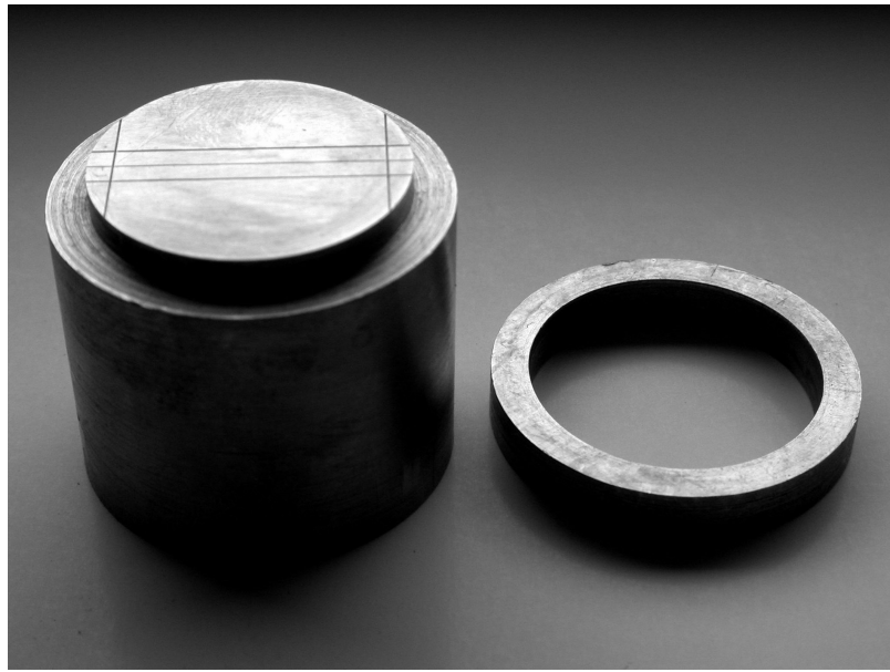
Figure 1. A round stainless steel test block with a stainless steel ring.
