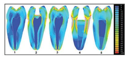
**Figure 3** Von Mises stress distribution of the five models.
