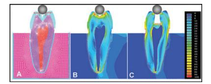
**Figure 2** 2D finite elements models. (A) Mesh of each area and load application; stress distribution and load application on sound (B) and prepared teeth (C).
