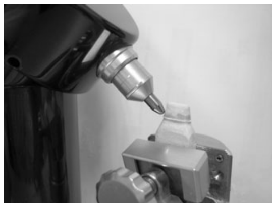
Figure 1 Procera AllCeram scanner with the die stone secured and ready for scanning.
