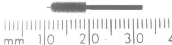
Figure 5 Photograph of the new bur (NEW). Courtesy of Diama Limited, London, UK. Dimension: mm.
