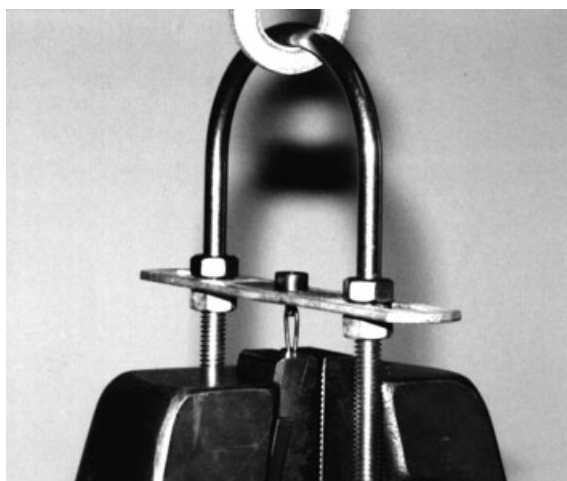
Figure 2 Custom specimen holding fixture mounted in the Instron Machine.
