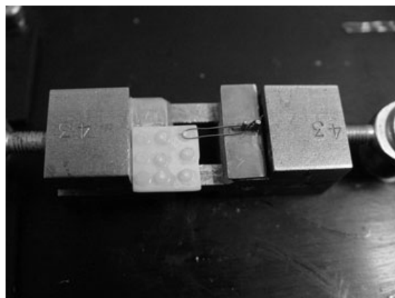
Figure 1 Specimen attached to the test machine.
