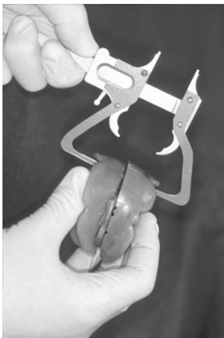
Figure 3 Measuring IAD with Boley gauge.
