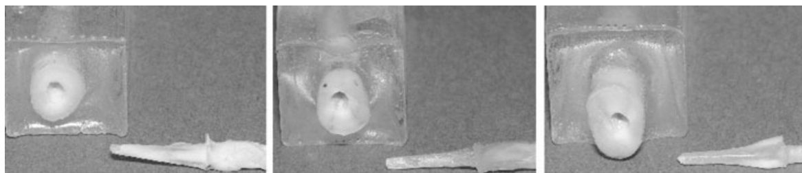
Figure 3 A comparison between the cement remaining on dislodged dowels representing the three groups. (A, left) An everStick dowel fabricated using the manufacturer's method. Note it is fully covered with luting cement after dislodgment. (B, center) An everStick dowel fabri-
