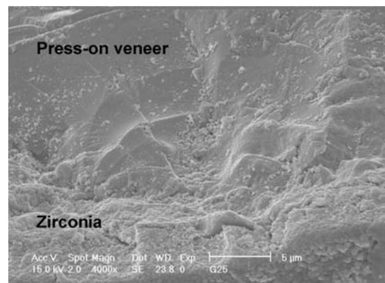
**Figure 2** SEM image of zirconia side of a broken double veneered microbar demonstrating an interfacial fracture. Fracture originated at zirconia press-on ceramic interface leaving exposed zirconia grains.
