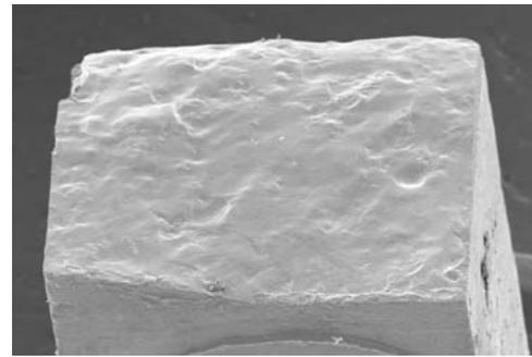
**Figure 1** SEM image of zirconia side of a broken microbar demonstrating a cohesive fracture. Fracture originated and propagated in the press-on veneer ceramic.
