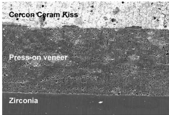
**Figure 3** Polished cross section demonstrating good contact between zirconia and press-on veneer and between press-on and layering veneer ceramics.
