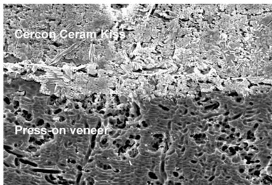
**Figure 4** Defect-free interface between the press-on and the layering veneer ceramics demonstrating different crystal and glass matrix structures.
