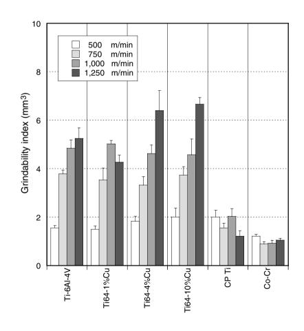
Figure 1 Grindability indexes (mm<sup>3</sup>) of metals tested.
