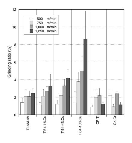
Figure 2 Grinding ratios (%) of metals tested.
