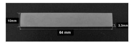
**Figure 2** Intact specimen for the flexural strength test.
