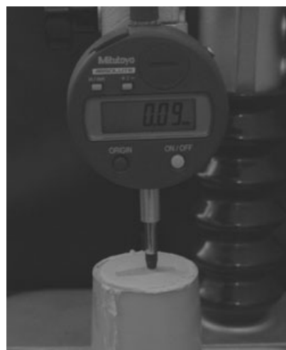
Figure 2 Dial comparator position for measurement of dimensional stability.
