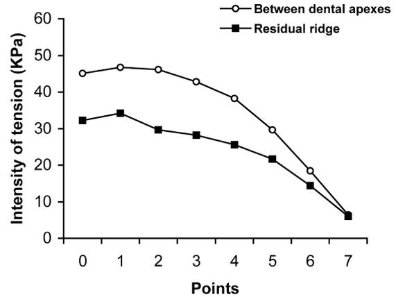
**Figure 11** Intensity of tension between dental apices and on the residual ridge after the application of uniformly distributed load on the circumferential retainer with long saddle.
