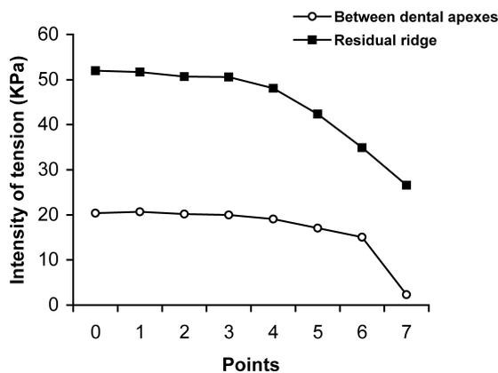
**Figure 10** Intensity of tension between dental apices and on the residual ridge after the application of load on the last artificial tooth (RPI retainer with short saddle).
