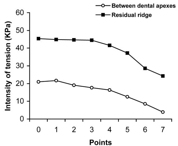
**Figure 12** Intensity of tension between dental apices and on the residual ridge after the application of load on the last artificial tooth (circumferential retainer with long saddle).
