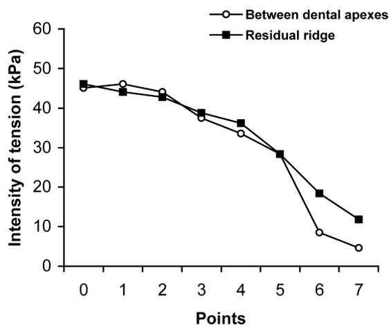
**Figure 13** Intensity of tension between dental apices and on the residual ridge after the application of uniformly distributed load on the circumferential retainer with short saddle.
