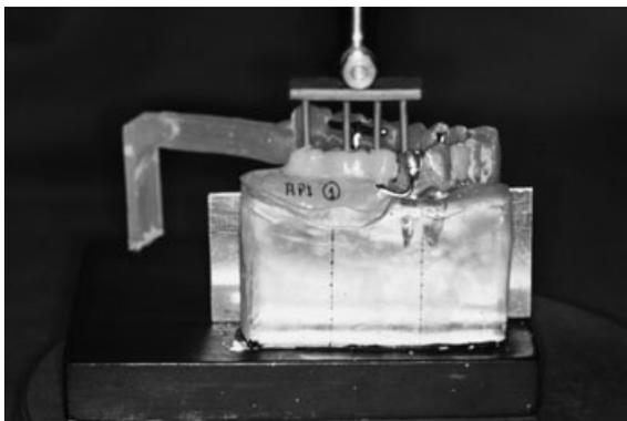
**Figure 2** Photoelastic model with the load application system.
