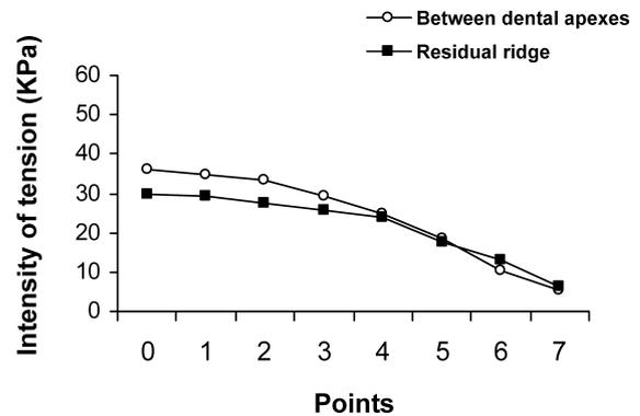
**Figure 3** Intensity of tension between dental apices and on the residual ridge after the application of uniformly distributed load on the T-bar retainer with long saddle.
