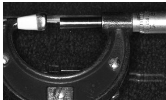
Figure 1 Experimental device permitting controlled introduction of marginal gap between prepared tooth and crown, in 25 \mu\text{m} increments.
