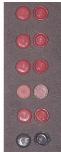
Figure 4 Examples of Locator attachments after soaking in their respective solutions and testing on the universal testing machine.
