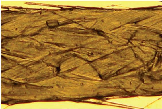
**Figure 3** Glass fibers (20× magnification).
