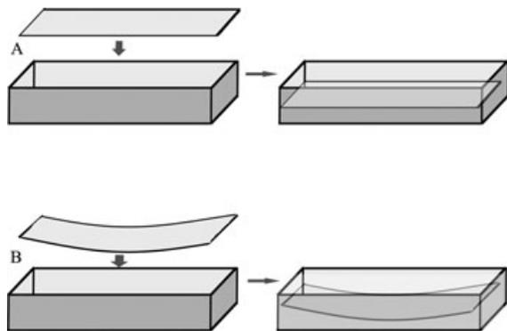
**Figure 1** Mold and two indexes used to orient the fibers in the desired position and curvature. (A) Mold, straight polyethylene index, and orientation of index for straight fiber position; (B) mold, curved polyethylene index, and orientation of index for curved fiber position.
