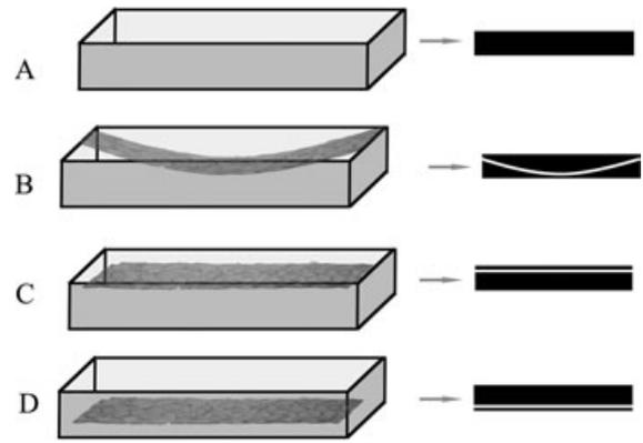
**Figure 2** Longitudinal cross-sectional design of the specimens and the resulting pictograms. (A) No fiber reinforcement; (B) fiber reinforcement in curved orientation; (C) in the compression side; (D) in the tension side.
