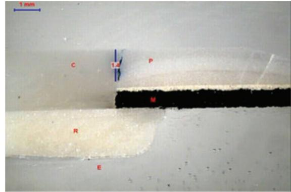
**Figure 7** Dye leakage at metal-ceramic/composite interface. P = Porcelain; M = Metal; C = Packable Composite; R = Vitrebond; E = Epoxy resin mold. Blue Bar = measurement of dye extension by millimeter (1 mm).
