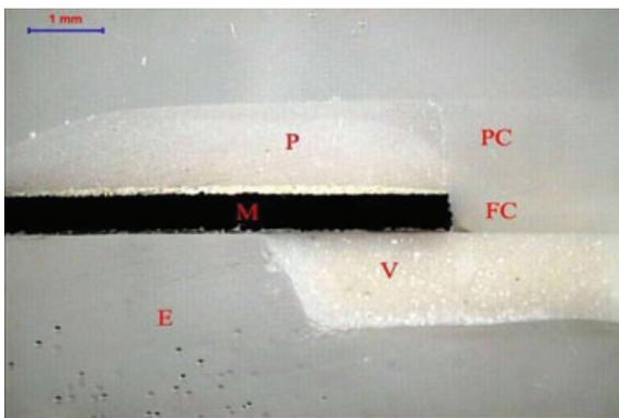
**Figure 6** No dye leakage at metal-ceramic/composite interface. P = Porcelain; M = Metal; PC = Packable Composite; FC = Flowable Composite; V = Vitrebond; E = Epoxy resin mold. Blue Bar = measurement of dye extension by millimeter (1 mm).
