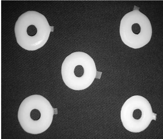
**Figure 1** Simulated metal-ceramic specimens.
