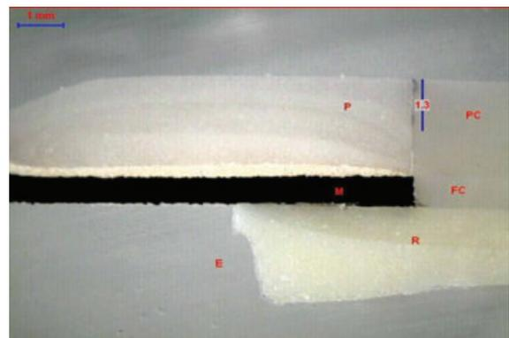
**Figure 8** Dye leakage at metal-ceramic/composite interface. P = Porcelain; M = Metal; PC = Packable Composite; FC = Flowable Composite; R = Vitrebond; E = Epoxy resin mold. Blue Bar = measurement of dye extension by millimeter (1 mm).
