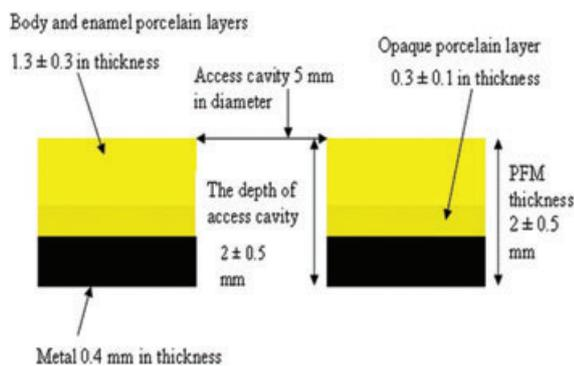
**Figure 2** Dimensions of simulated metal-ceramic specimens.
