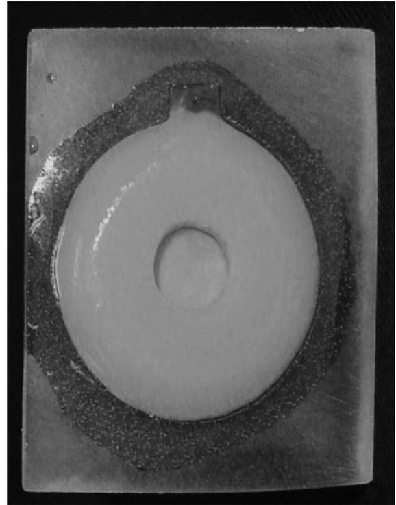
**Figure 3** Specimens and epoxy-filled cavity fixed using glue and epoxy resin.
