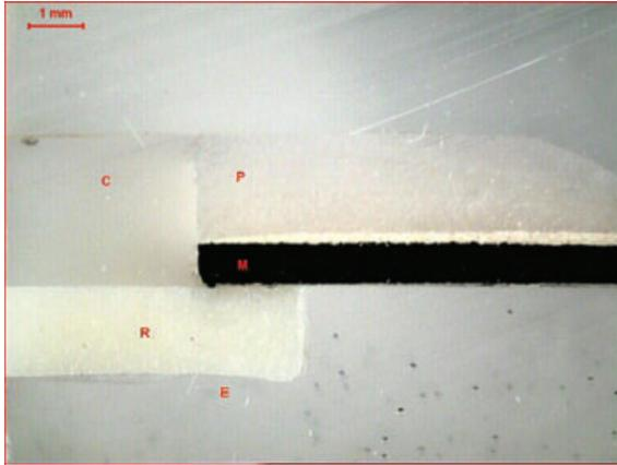
**Figure 5** No dye leakage at metal-ceramic/composite interface. P = Porcelain; M = Metal; C = Packable Composite; R = Vitrebond; E = Epoxy resin mold. Red Bar = measurement of dye extension by millimeter (1 mm).
