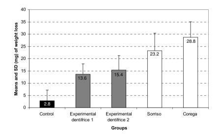
**Figure 1** Means and standard deviation weight loss of specimens after brushing with groups of dentifrices. Columns with identical colors were not significantly different.
