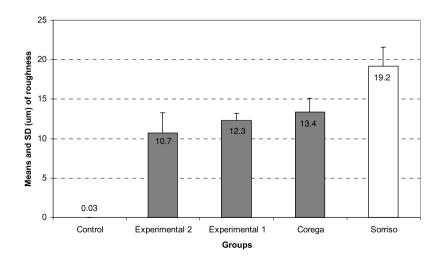
**Figure 2** Means and standard deviation of dentifrice roughness of the specimens after brushing. Columns with identical colors were not significantly different.
