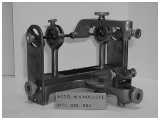
Figure 9 The Model M Kinoscope of 1923 had an early vintage incisal guide table and wide but thin outside posts. (courtesy Teledyne-Hanau factory collection).
