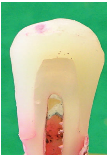
Figure 7 Composite resin crown cemented with Panavia F 2.0. This specimen was given a score of 2. The die penetrated along the interface and reached a level limited to the lower half of the axial wall.
