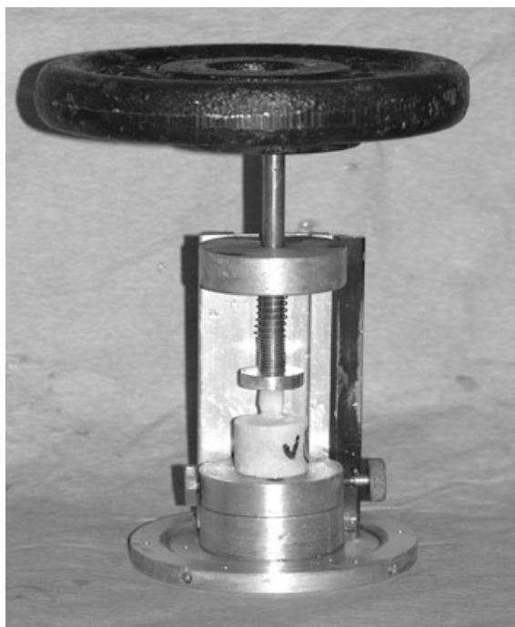
Figure 3 Cemented crown seated in a device with constant occlusal load of 5 kg maintained until initial setting was achieved.
