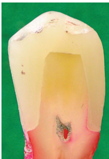
Figure 8 Composite resin crown cemented with RelyX Unicem. This specimen was given a score of 2. The die penetrated along the interface and reached a level limited to the lower half of the axial wall.
