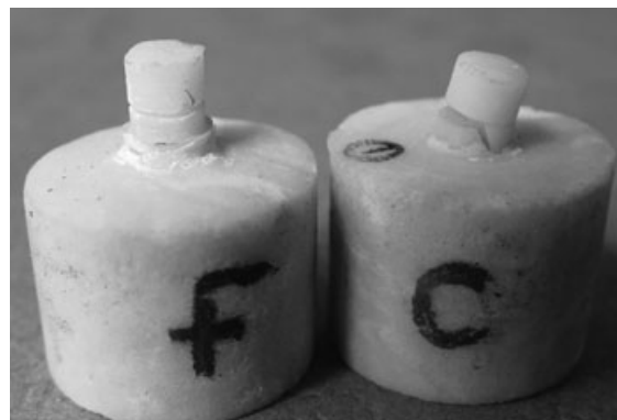
Figure 2 Representative specimens demonstrating the fracture patterns for fiber dowel (F) and ceramic dowel (C).
