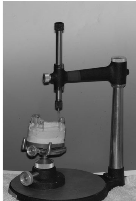
Figure 7 Dental surveyors led to the development of advanced RPD concepts such as guiding planes.
