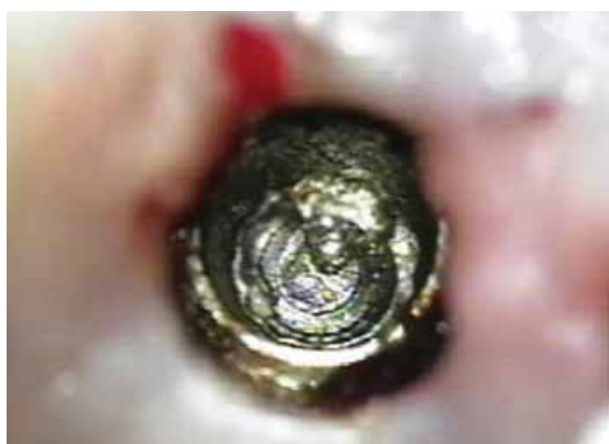
Figure 2 Fractured abutment screw seen through surgical microscope.
