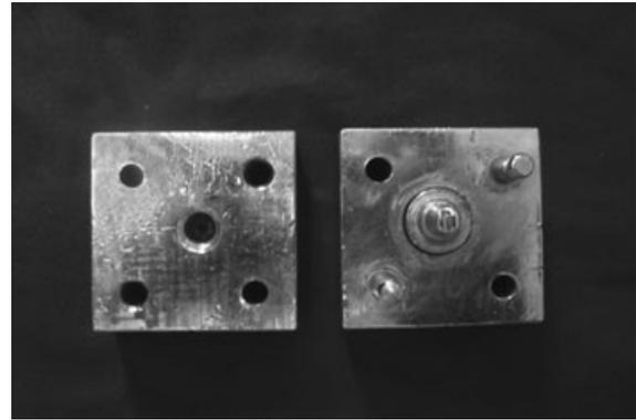
**Figure 1** Stainless steel metal die (die and counterpart).
