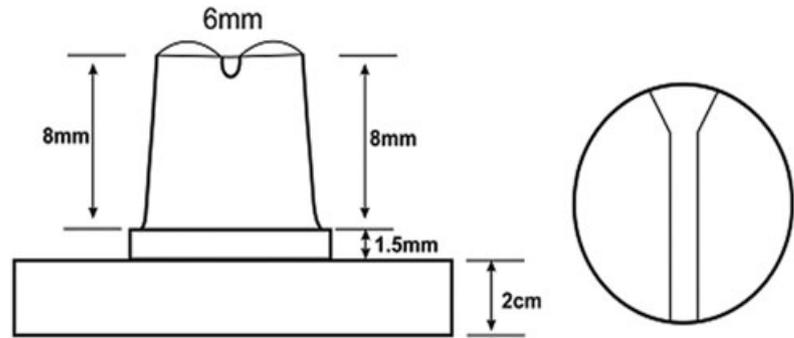
**Figure 2** Schematic representation of metal die. Circle shows the “Y” index line.
