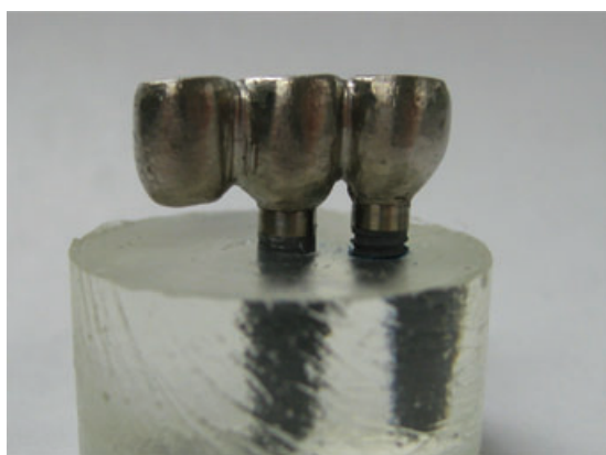
Figure 10 Specimen assembled in resin medium.
