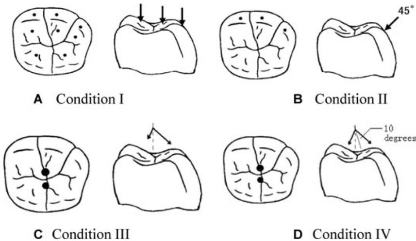
**Figure 1** Loading conditions of the all-ceramic crown. (In Conditions I, III, and IV, a total of 600 N bite force was applied, while in Condition II, 255 N masticatory force was applied.) (A) Condition I, (B) Condition II, (C) Condition III, and (D) Condition IV.
