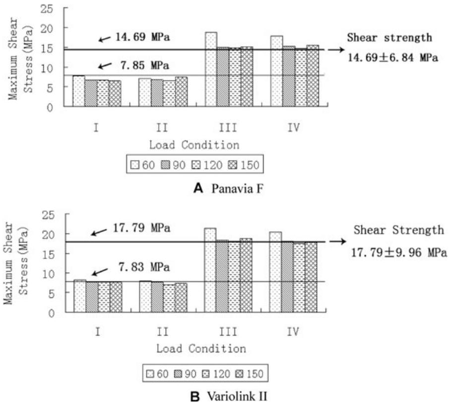
Figure 5 Maximum shear stress in the cement. (A) Panavia F and (B) Variolink II.
