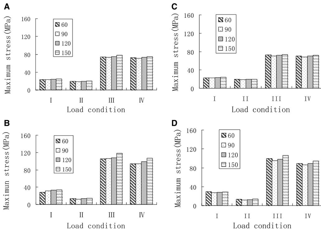
Figure 6 Comparisons of the maximum principal stress with the cement thickness (in μm) in the four loading conditions. (A) Stress at the upper surface of the veneer, Panavia F; (B) Stress at the lower surface of the core, Panavia F; (C) Stress at the upper surface of the veneer, Variolink II; (D) Stress at the lower surface of the core, Variolink II.
