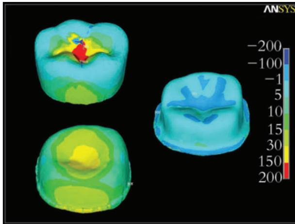
**Figure 3** Stress distribution in the veneer, core, and cement when the crown is subjected to loading Condition IV.
