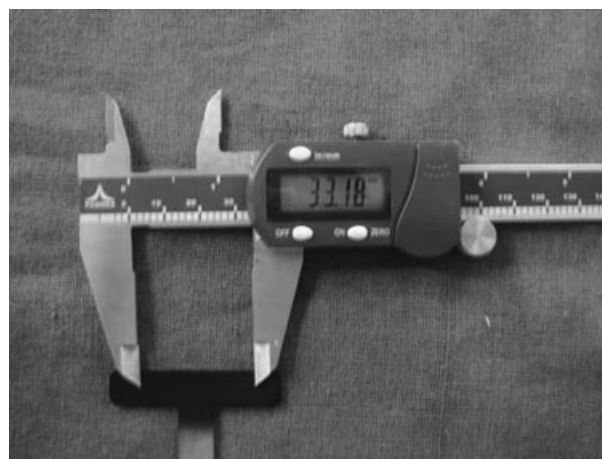
Figure 6 Measurement of intercanine distance with digital vernier caliper.
