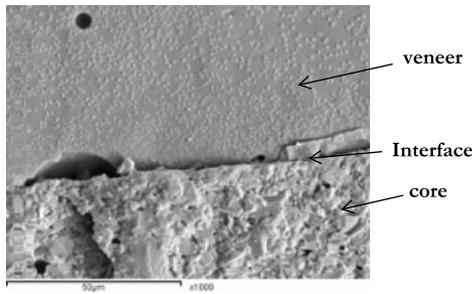
**Figure 1** SEM of failed Vitadur-N-veneered crown showing the coarse, granular nature of its veneering material. In-Ceram core shows dense alumina particles of different shapes, sizes, and arrangement embedded in a nonporous matrix. Porosities and gaps are apparent at the core/veneer boundary showing incomplete adherence and debonding of the porcelain from the core surface.
