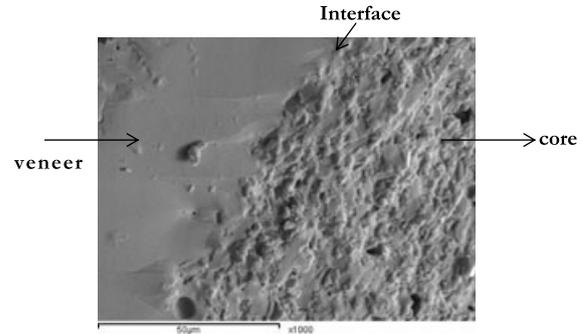
**Figure 2** SEM of failed Vitadur- $\alpha$ -veneered crowns showing distinct morphology from the earlier generation. The particle size of the veneering material is fine textured and interlocks intimately to the alumina core. The interface appears defect-free, suggesting a good bond between the veneer and the core.
