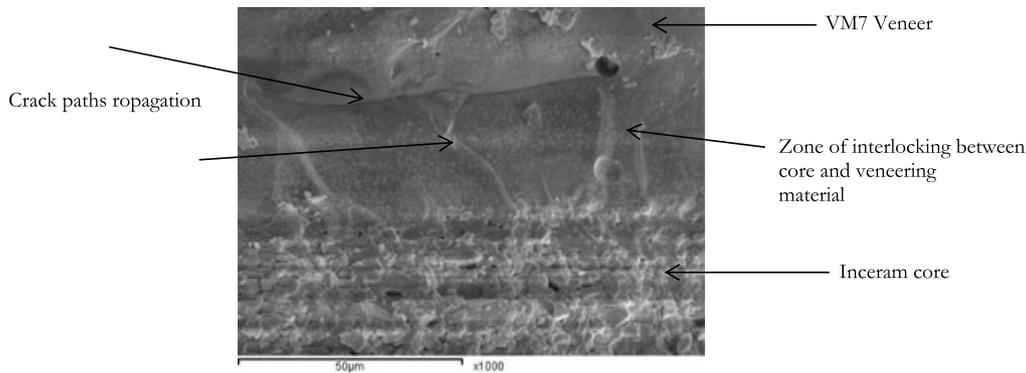
**Figure 3** SEM of failed VM7 crown showing interlocking between the alumina core and veneer, creating a zone where the materials appear to blend and intertwine, making them not clearly identified from each other.
