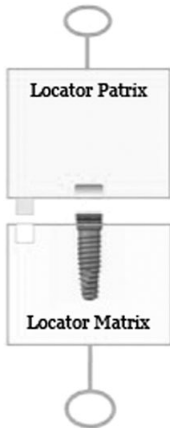
Figure 1 The acrylic resin cylinders used for testing pink Locator attachments. The first acrylic resin cylinder has a metal housing with a Locator matrix embedded within. The second acrylic cylinder has a Locator patrix abutment attached to implant.
