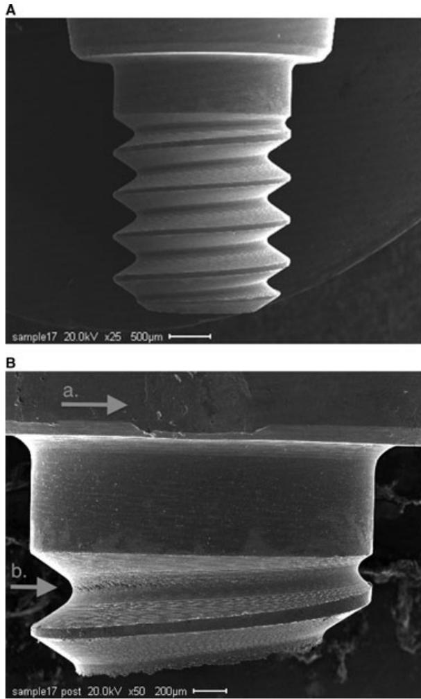
**Figure 5** (A) Group 1 implant pre-fatigue cycling and prefracture. (B) Group 1 implant post-fatigue cycling and postfracture. Arrow “a” indicates the facet formed prior to fracture, while “b” demonstrates ductile delamination following screw loosening.
