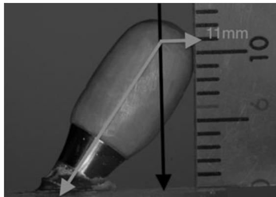
**Figure 1** Implant/abutment complex embedded in acrylic according to ISO 14801 guidelines with wax-up of loading member in position.
