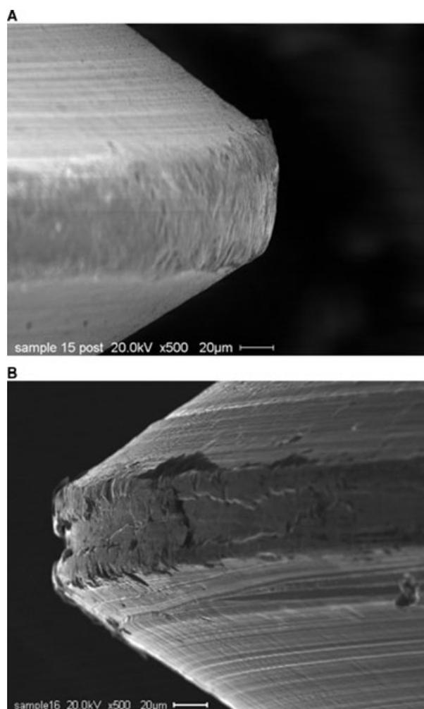
**Figure 4** (A) Group 1 first thread in profile. Note smooth, rounded surface. (B) Group 2 first thread in profile. Note rough surface.
