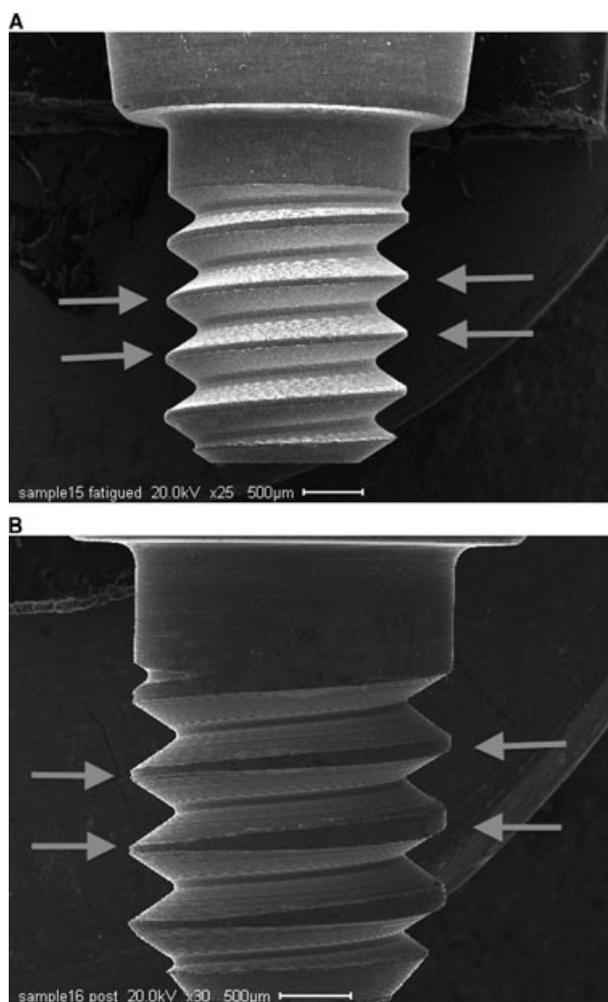
**Figure 3** (A) Group 1 abutment threads in profile. Note arrows pointing out thread profile. (B) Group 2 abutment threads in profile. Note arrows pointing out thread profile.
