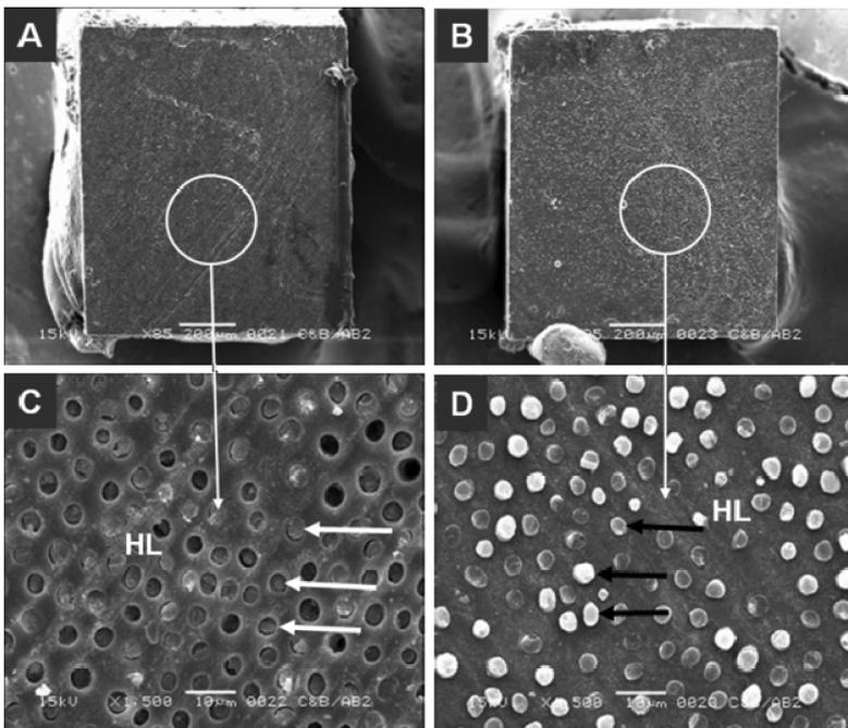
**Figure 4** SEM fractography analysis of C&B Cement/All-Bond 2 (24 hours). In A and B, opposite sides of the same fractured specimen are observed, illustrating type II fracture pattern (85 $\times$ ). C and D present, at higher magnification, images of the circled areas in A and B, the morphologic aspect of the cohesive fracture in the hybrid layer (HL), precluded dentin tubules (white arrows) and fractured fragments of the resin extensions (black arrows) can be observed (at 1500 $\times$ ).
