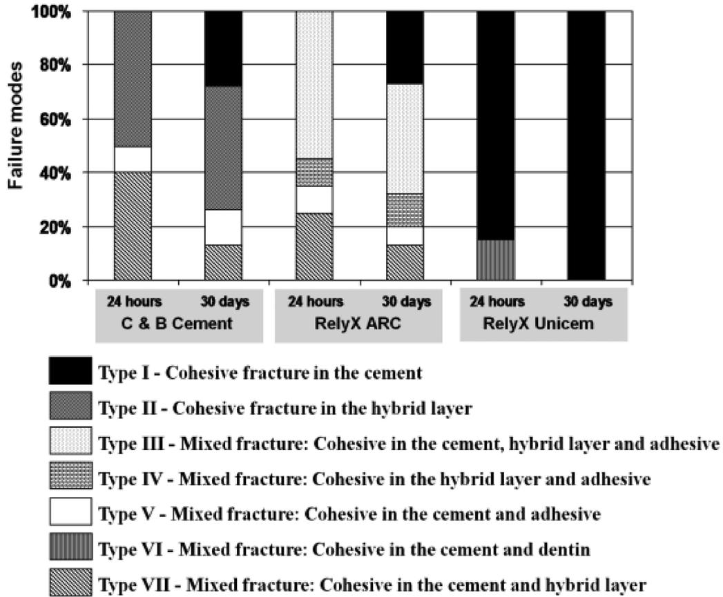
**Figure 1** Proportional prevalence of failure modes after microtensile bond strength testing for all experimental groups after 24 hours and 30 days.
