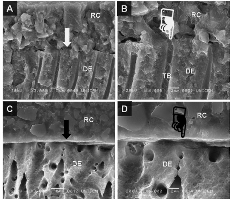
**Figure 5** SEM photomicrograph of RelyX Unicem bonded to dentin. A (3000×) and B (6000×) (fractured specimens) exhibit an intimate contact of the resin cement with the dentin tissue (white arrow); dentin tubules (TB) with no resin infiltration (white hand) were noticed. In C and D (conventionally processed specimens), images show a non-authentic hybrid layer (black arrow) and also the interaction between the resin cement and the dentin (black hand). RC—resin cement; DE—dentin.
