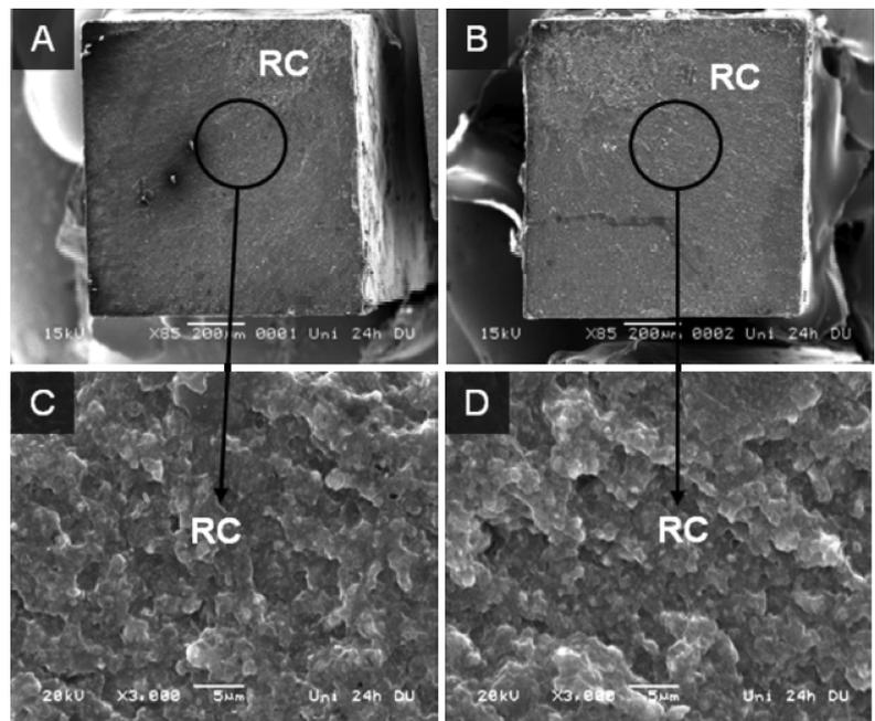
**Figure 2** Photomicrography images of RelyX Unicem at 24-hour evaluation time. In A and B, opposite sides of a fractured specimen illustrate type I fracture pattern (85×). C and D represent the circled regions in A and B at higher magnification. The morphological aspect of a fractured region of the RelyX Unicem cement, in which a dense resin matrix with no porosity involving the inorganic fillers, is observed. The characteristic morphology is demonstrated (3000×). RC—resin cement.
