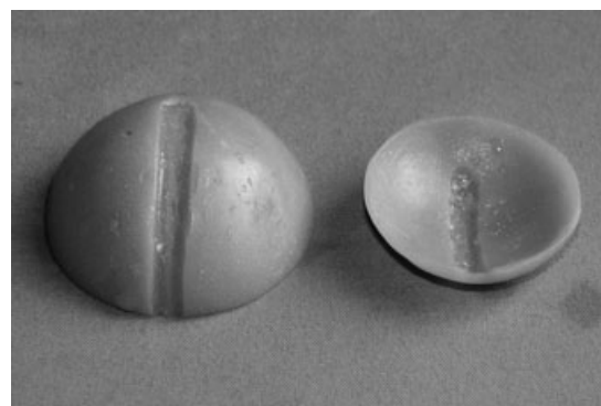
Figure 4 Grooves made on concave surface of the smaller and convex surface of the bigger hemispherical resin plates to accommodate the curvilinear zigzag portions of the coil.
