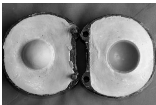
Figure 2 Hemispherical heat-polymerizing acrylic resin plate fabricated from the gypsum mold.
