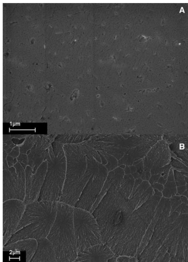
**Figure 6** SEM images of the Lucitone 550 denture base resin with no silver nanoparticle. (A) polymer surface and (B) polymer fracture surface. Magnification (A) 25,000 $\times$  (B) 5000 $\times$ .
