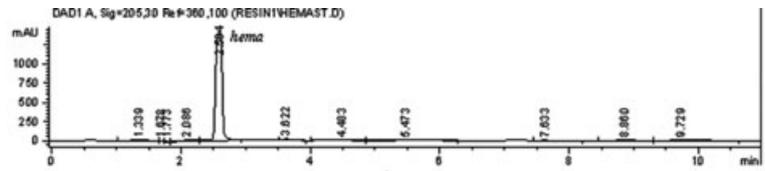
**Figure 2** Standard peak and retention time of HEMA.
