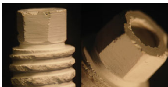
Figure 1 Zirconia implant design with external hex implant head.
