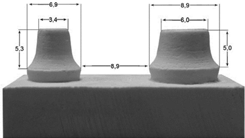
**Figure 1** Master model and its measurements; 120° chamfer preparation and a convergence angle of 15°.
