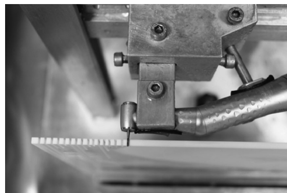
Figure 4 Cutting test performed on the machinable glass ceramic (Macor).
