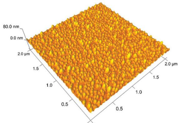
**Figure 2** AFM image showing the film topography used Gag. Note the regular distribution of Ag-NPs (peaks) throughout the film surface.**Table 2** Results of one-way ANOVA for comparison of *C. albicans* counts (cfu/specimen), Ra and Rz parameter data (\* $p < 0.05$ )
