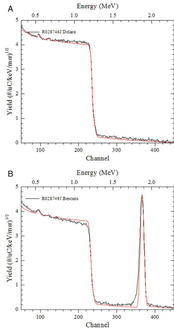
**Figure 1** RBS (black) of films used in (A) Gdlc and (B) Gag and simulation (red) performed to characterize the elemental chemical composition (energy, x-axis) and thickness of films (measured by the energy width of the C peak divided by the energy loss of the incident ion particle per unit depth). Note the presence of a peak of carbon ( $\sim 0.5 \text{ MeV}$ ) to both spectra and the peak of silver ( $\sim 1.9 \text{ MeV}$ ) to Gag. The y-axis is related to counts of atoms.
