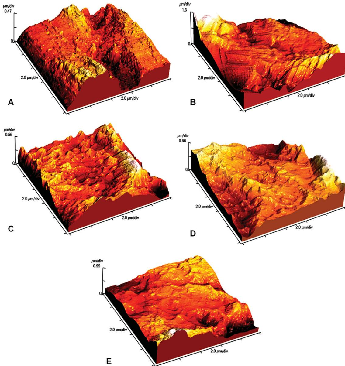
**Figure 1** AFM images of cp Ti plates: (A) Machined control; (B) Airborne-particle abrasion; (C-E) Experimental hot-etching solution applied for 15, 30, and 60 minutes, respectively.
