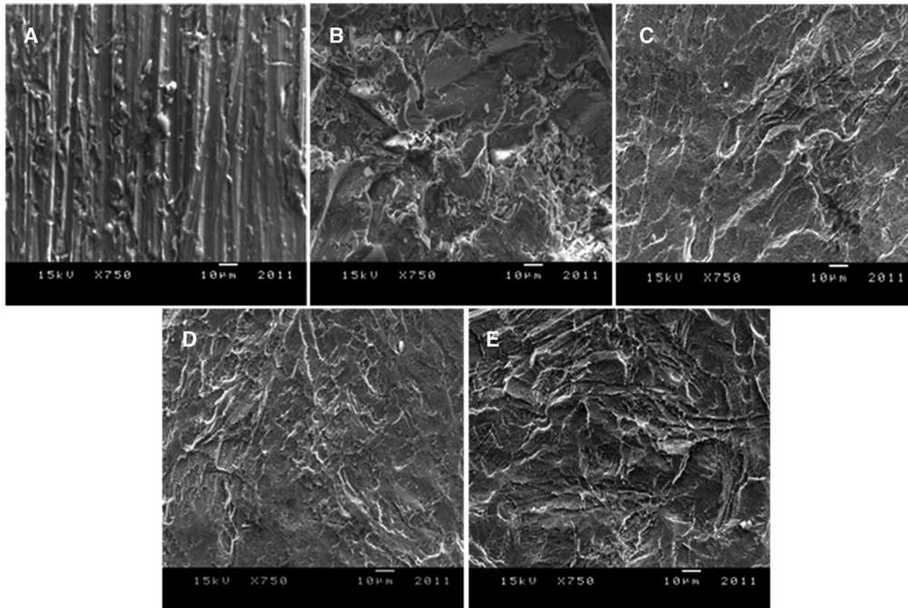
**Figure 2** SEM photomicrographs of cp Ti plates: (A) Machined control; (B) Airborne-particle abrasion; (C-E) Experimental hot-etching solution applied for 15, 30, and 60 minutes, respectively.
