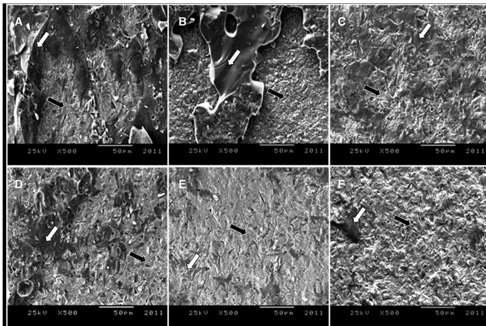
**Figure 3** Representative SEM photomicrographs of the peeled surface of cp Ti/veneering porcelain system: (A-D) Mixed bond failure for cp Ti/DK (etching for 30 minutes), cp Ti/VT (etching for 15 minutes), cp Ti/ST (etching for 60 minutes), and cp Ti/DK (etching for 60 minutes)
